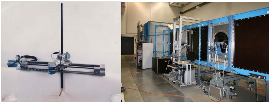
Figure 2. Traverse mechanism example Ref. [3], and the wind tunnel facility at TU Braunschweig
