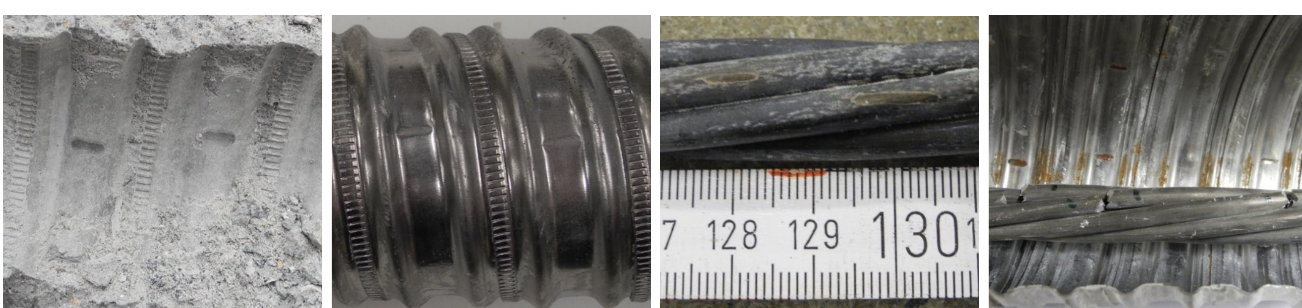
Effects of Lateral Pressure on Concrete (left), on the Duct (middle left) and on the Prestressing Steel (middle right) as well as resulting Wire Fractures (right)
