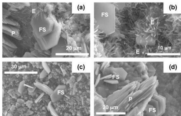
Fig.1 The dissolution of the calcium hydroxide (P), and the forming of Friedel's salt (FS) [3]
