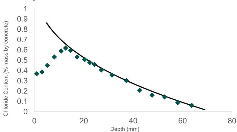
Fig.2: Typical simplified model for diffusion of chloride (solid line) vs. field samples, deviation is due drying/wetting cycles (max. concentration is not on the surface)[1]
