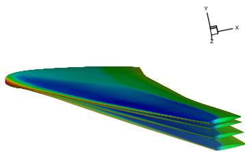
Convergence to stationary aeroelastic state for transonic flow.
