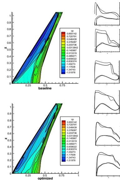
Pressure distribution on the baseline and optimized geometries - drag reduction with constant lift taking into account aero-elastic coupling, 240 shape design variables, coupled adjoint approach.
