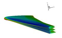
Convergence to stationary aeroelastic state for transonic fbw.
