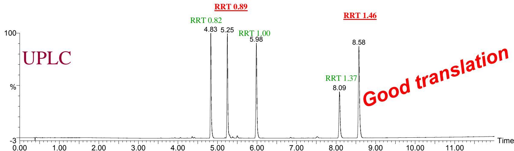
Generic UPLC method (12mins) 40°C 100x2mm Gravity C18 1.7µm
