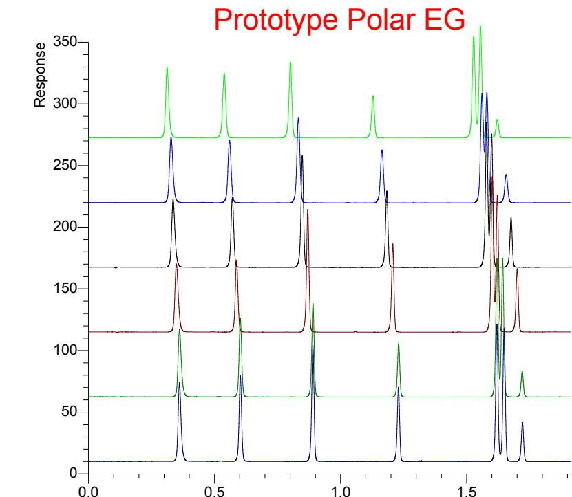
Overlaid gradient separation of Waters neutral SST after multiple series of 200 injections
