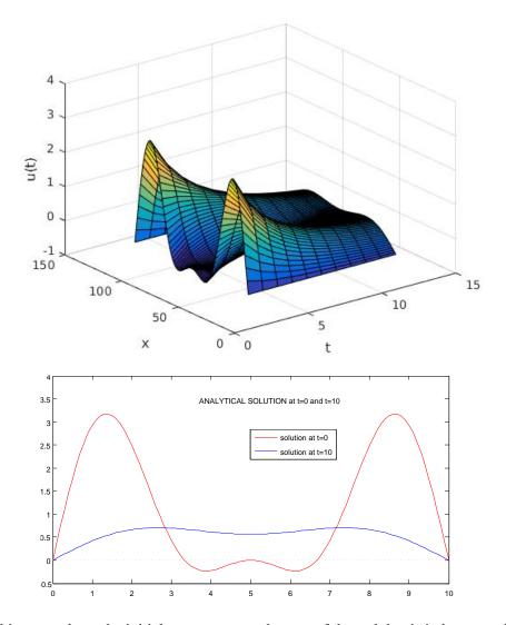
The two bigger peaks at the initial state warm up the part of the rod that is in between the peaks and the temperature is decreasing continuously in the bar. The peaks are almost completely smoothed down at T=10. Physically: Since there is no source term in the PDE, the temperatures should decrease over time. Hence the above obtained behavior corresponds to the physically expected one.
