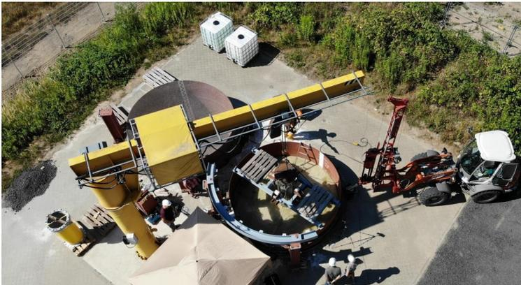
**Figure 5-1: Geotechnical test pits and infrastructure at IGG-TUBS during installation of model pile (test Z03, pile installation)**
