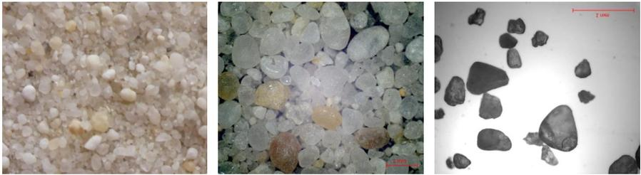
Figure 5-4: Macroscopic (left) and microscopic (middle, right) view of model sand
