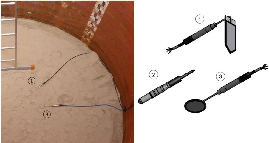
**Figure 5-10: Earth pressure sensors in the test pit (left) and detail of earth pressure spade ① pore water pressure transducer ② and earth pressure pad ③ (right, by courtesy of Glötzl)**
