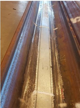
**Fig. 8: Covered and waterproofed strain sensor line ready for field deployment.**
