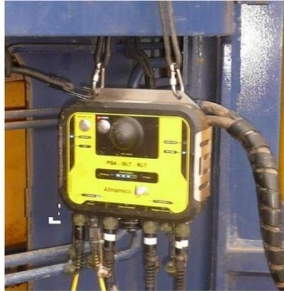
Figure 4: The Allnamics PDR-system, which collects and stores the raw data and transmits it wireless to the field laptop
