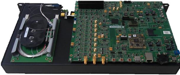
FAZ I4 Interrogator, optics (left) and electronics (right) boards
