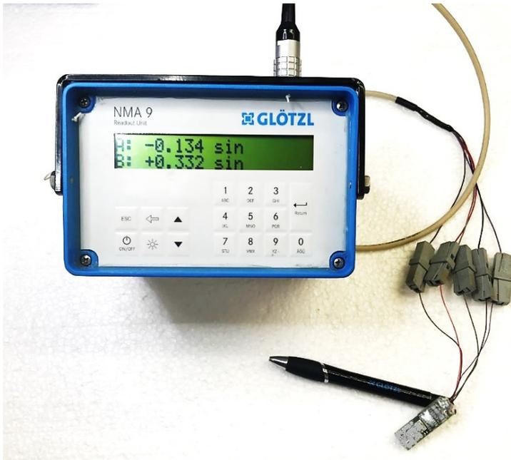
**Fig. 14-** Glötzl hand-held readout unit for inclination sensors connected to the MEMS
