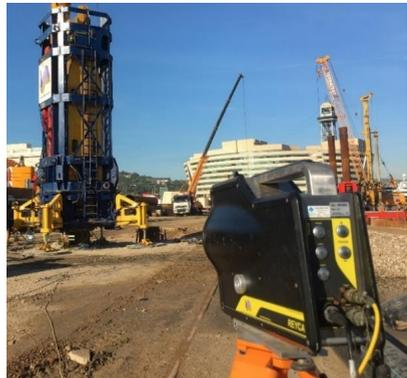
Figure 3: The displacements are measured with the Reyca Optical System
