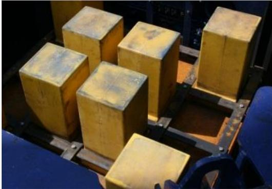
**Figure 6: The spring set up can be adjusted in stiffness to get optimal load and load duration**
