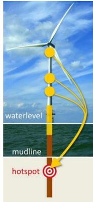
**Figure 7 : Concept of virtual sensing, using sensors on the top structure strain histories and fatigue progression are estimated on any virtual sensor location**
