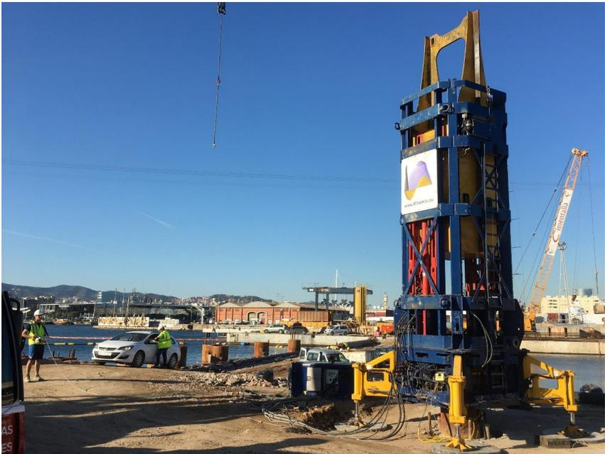
Figure 2. StatRapid Device ready for testing on site
