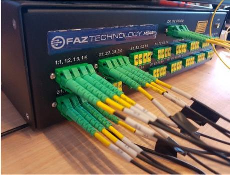
**Fig. 4:** FAZ 64 channel interrogator, using an optical multiplexer system.
