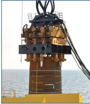
APE Holland supplies vibratory hammers and hydraulic power units, which can be used for vibrating sheet piles and tubular piles. The wide range of equipment can be used for driving small sheet pile walls as well as the largest piles for offshore wind farms, both onshore as offshore.
