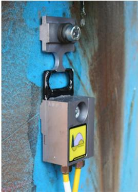
Figure 8, Combined acceleration/strain transducer for VDA
