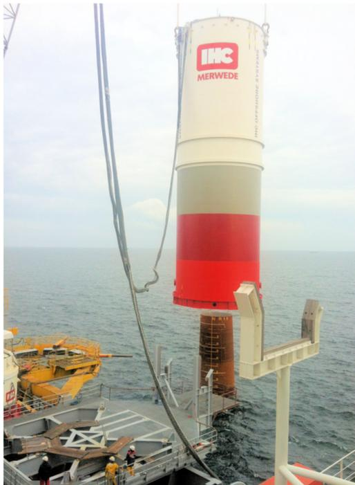
Figure 5, NMS for impact pile driving
