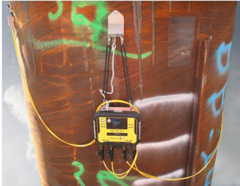
Figure 9, PDR monitoring unit with Wi-Fi signal transmission for VDA
