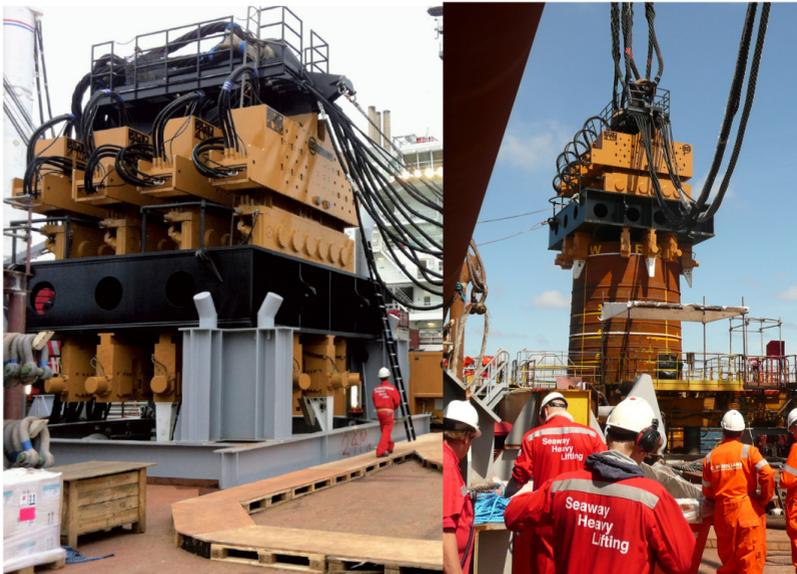
Figure 3, SQK on deck and vibratory driving of monopile with SQK
