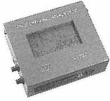
**Pile Driving Analyzer®-PAL**
