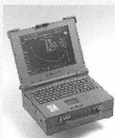
Statnamic measuring system (FPDS)
