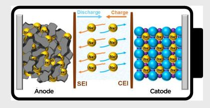
The current project aims to a systematic study of polymer electrolytes with sodium-ion based on preliminary promising data that showed at low temperature an ionic conductivity higher than the PEO-Li based electrolyte.
