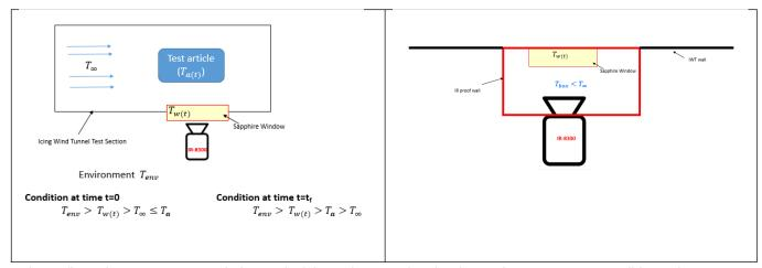
The reflected temperature and the emissivity value set for the hot substrate are not valid as the substrate is cooled below the window temperature. To improve the measurement, it is planned to build IR shielded box around the lens and the window and maintaining the temperature inside the box lower than the temperature of the wind tunnel as shown below. Thereby, minimizing the reflected temperature.
