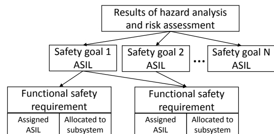
Fig. 4. Relation of HARA, safety goals and functional safety requirements according to [6].
