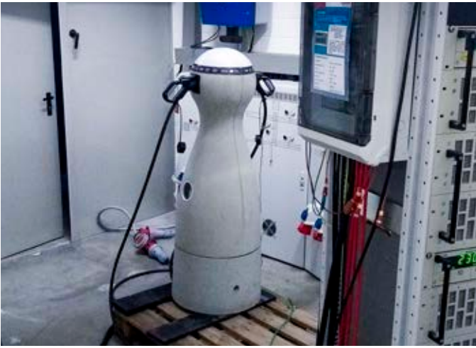
PION AG charging station in the 7-hour 44 kW continuous load test
