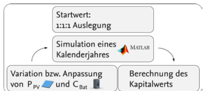
Figure 2: Iterative process to determine an economic optimum for PV system and storage system
