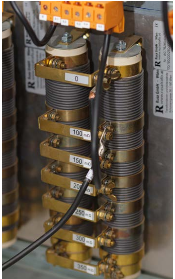
Conductor emulating elements equivalent to up to 1.8 km of low voltage cable
