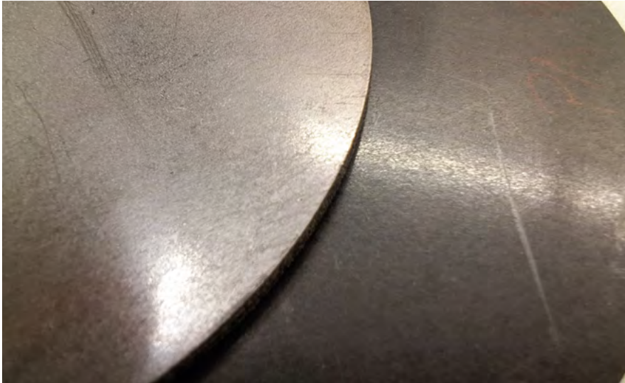
Metallised plastic samples for improved measurement accuracy through vapour-deposited electrodes
