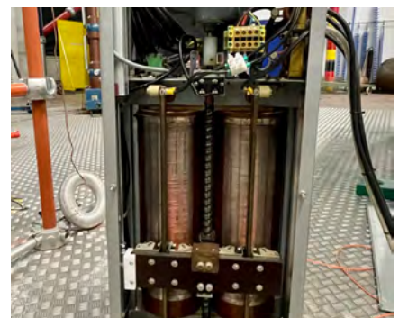
Figure 3: Positioning transformer with absolute value encoder
