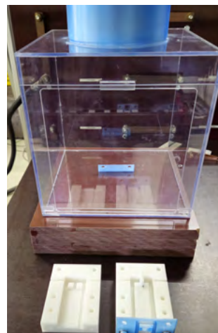
Figure 5: Switch chamber with extraction for material testing
