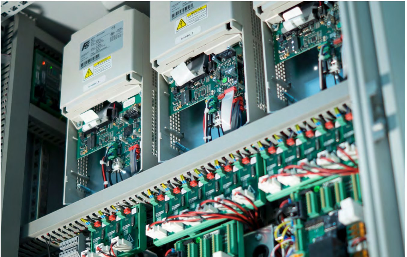
Figure 3: Fully programmable three-phase prototype inverter
