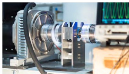
30 kW COUPLED MACHINE SET (ASYNCHRONOUS MACHINE AND SYNCHRONOUS MACHINE)
