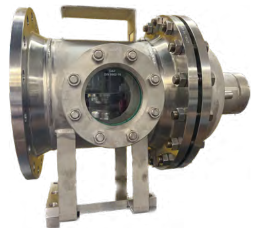
Figure 2: Test container for examination under various environmental conditions
