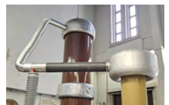
Figure 7: High-voltage connection of an 800 kV transformer
