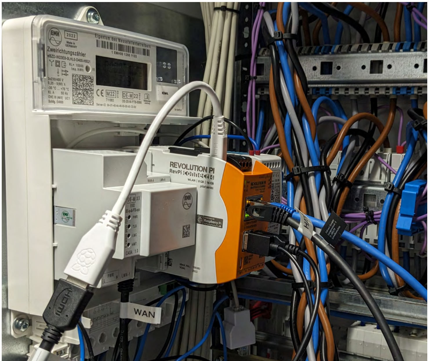
Figure 2: Smart meter with HEMS prototype in laboratory environment.
