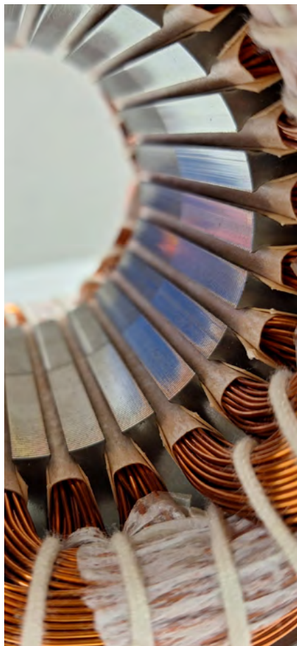
Figure 6: insulation system for electromobility, Maik Kahn
