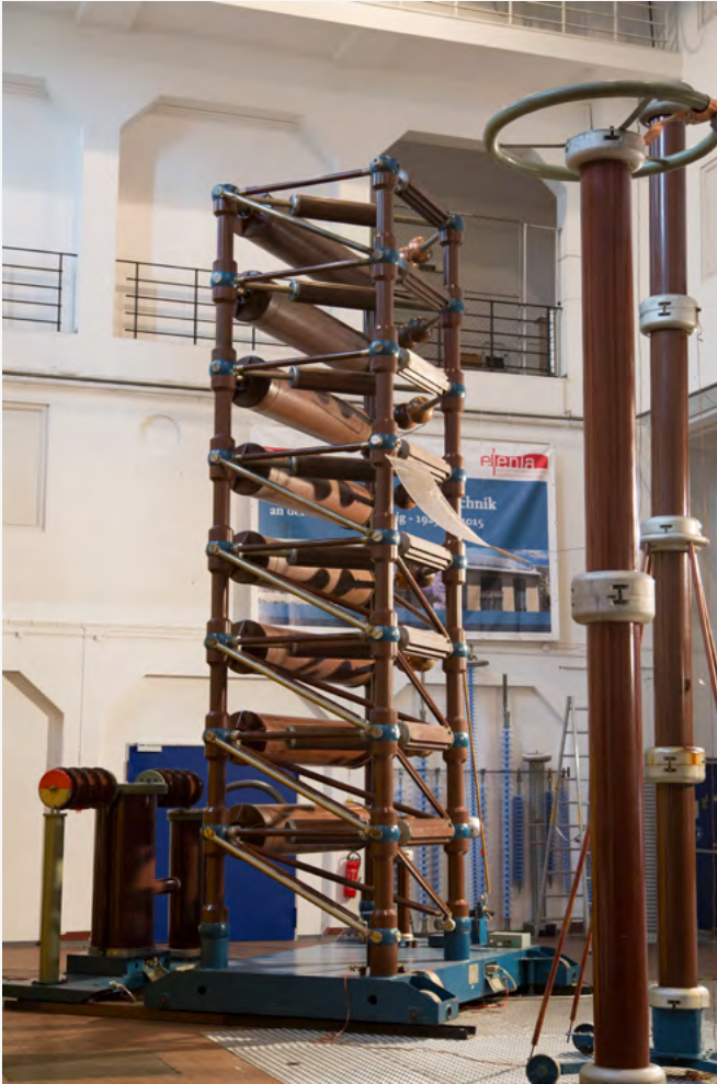
IMPULSE VOLTAGE GENERATOR
