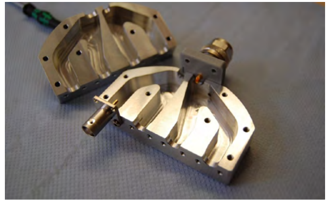
CNC-milled housing for a measuring adapter
