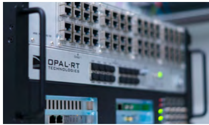
Figure 3: OPAL real-time simulator with analog interfaces for controlling components in the laboratory
