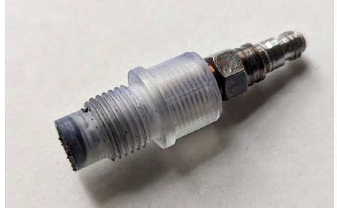
SLA 3D printing of an adapter for mounting pressure sensors.
