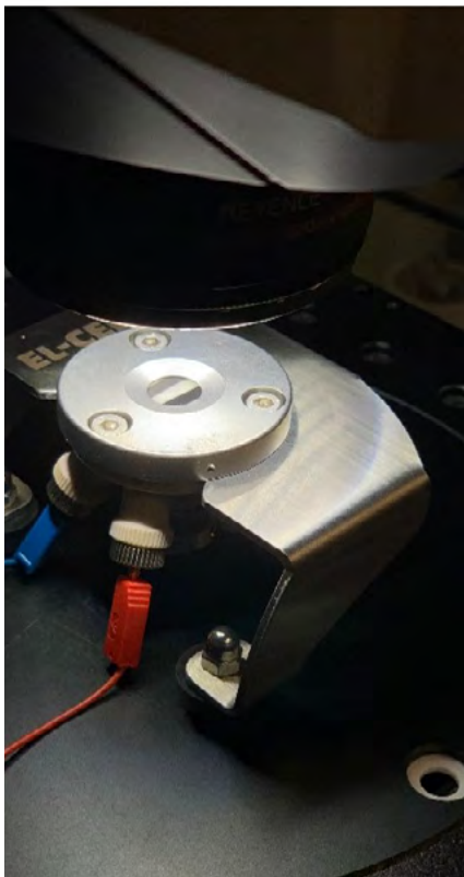
Figure 2: Optical battery cell for in-operando diagnosis of electrodes during formation
