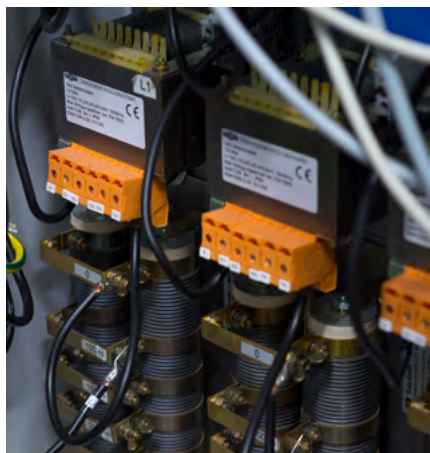
Figure 5: Line-replicating elements correspond to up to 1.8 km of low-voltage cable
