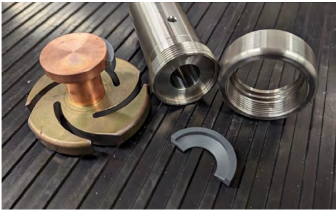
Manufacturing of an adapter from stainless steel to accommodate copper switch contacts
