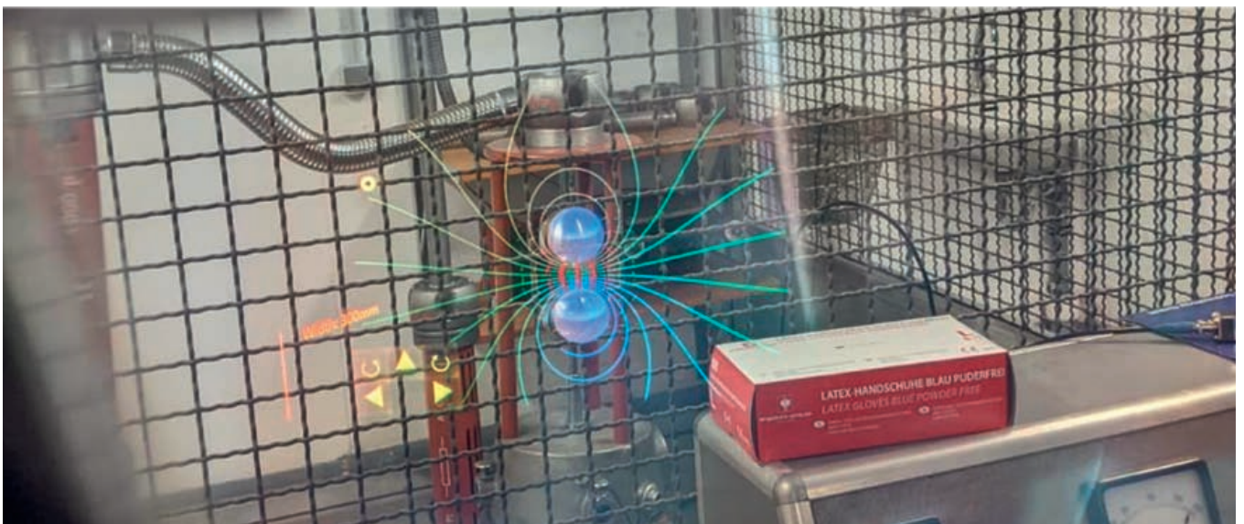
Figure 1: Risks of electric fields on a spark gap Figure 2: Photography through augmented reality glasses
