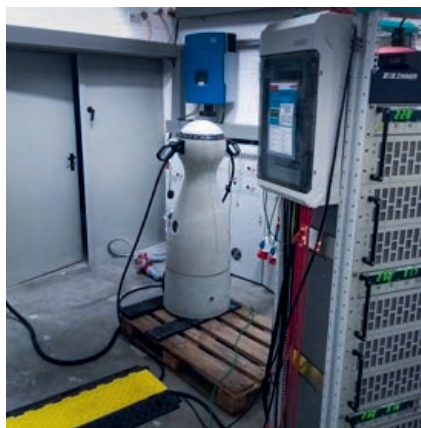
Figure 1: PION AG charging station in 7-hour 44kW continuous load test
