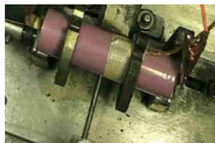
t = 126 ms after nail penetrated the can wall
