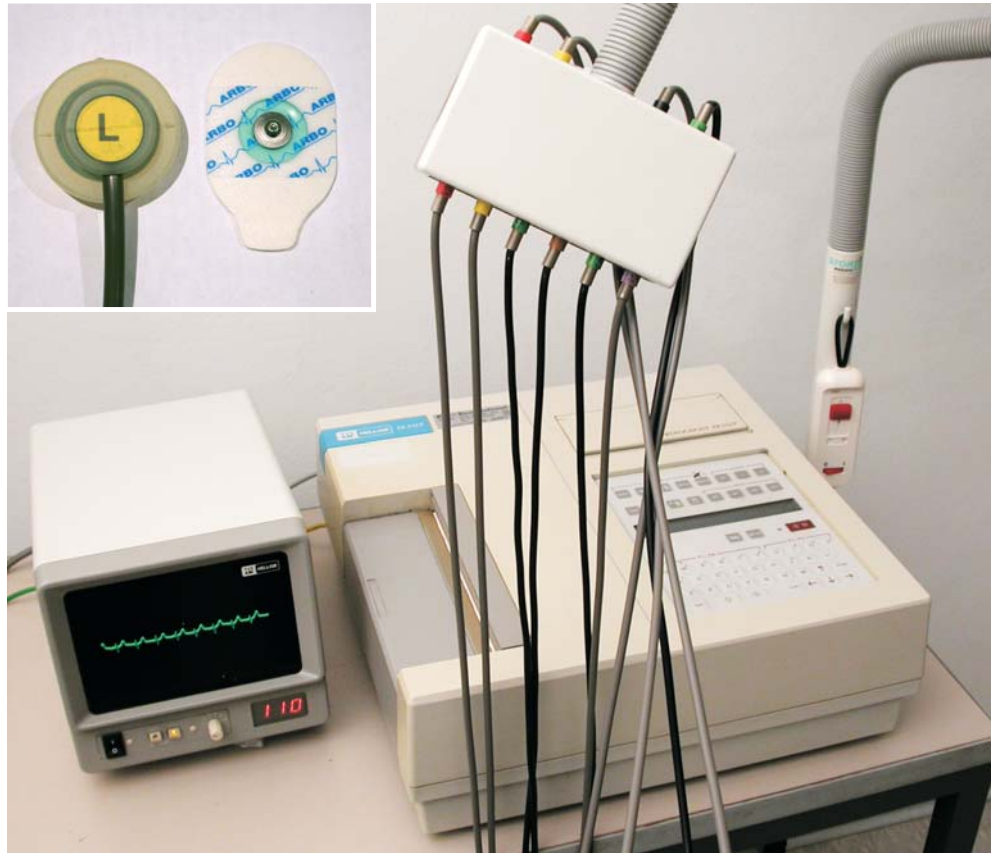
Suction and adhesive electrode of a conventional ECG system
