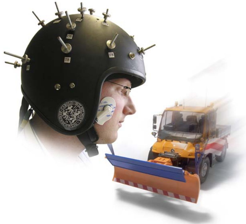
Electrode helmet for controlling a device, here a vehicle
