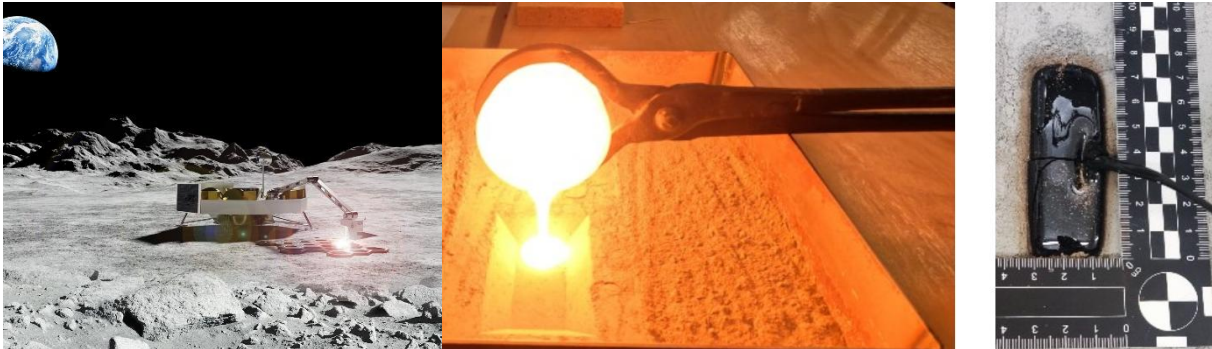
Fig 1: Lunar construction concept, regolith casting and obtained brick
