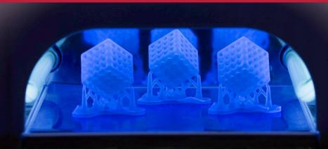
Two different post-curing sources are available. Both produce light and heat and various combinations of the parameters must be systematically investigated. The exact influence of UV-light exposure, temperature on properties must be understood. The best combination of parameters must be found and proven experimentally.
