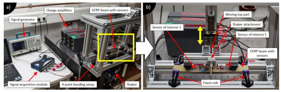
3D printed piezoelectric composites are characterized by measuring their piezoelectric coefficient d<sub>31</sub>. The measuring procedure shown above must be developed further. Sensors are glued on thin GFRP beam and are loaded with 4-point bending. Input and output data is measured and evaluated with Matlab. The reliability of this measuring method must be proven experimentally with different sensors, i.e. different sensor adhesion techniques and placements on the GFRP beam.
