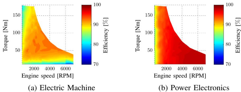
**Figure 5** – Efficiency maps and thermal power losses within the powertrain [9]
