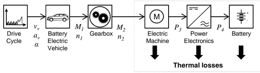
**Figure 4** – Overview drivetrain model
