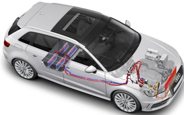
**Figure 1** – Typical thermal management system for an electric vehicle
