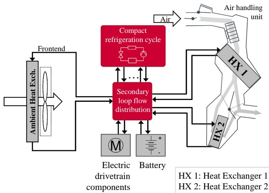
**Figure 2** – Thermal management using a compact refrigeration cycle and secondary loop flow distribution unit
