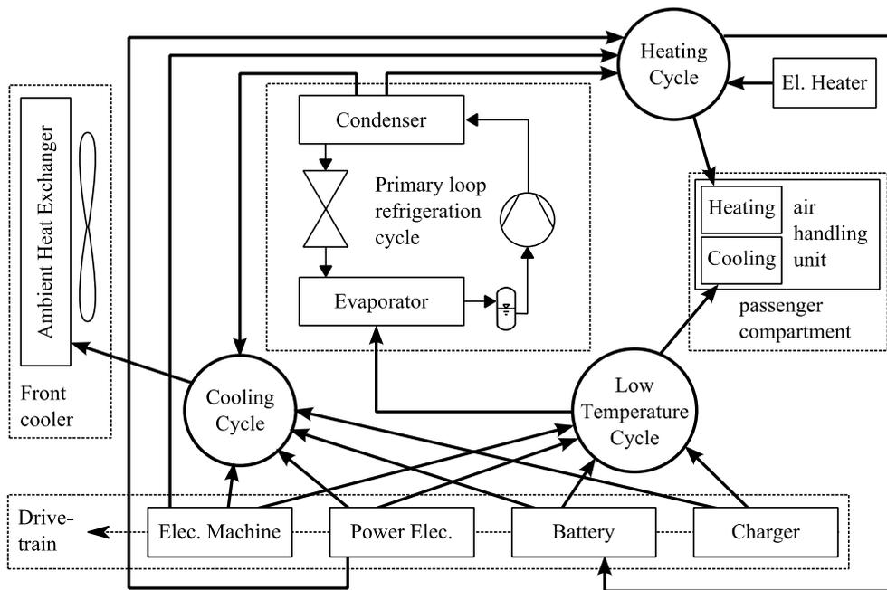
**Figure 6** - Possible energy flows between components and coolant cycles
