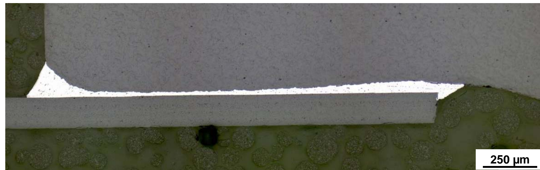
ceramic-ceramic joint realized with reactive air brazing
