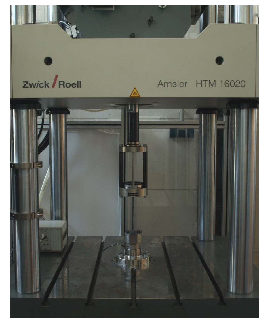
high speed testing machine with implemented clamping devices for tensile tests
