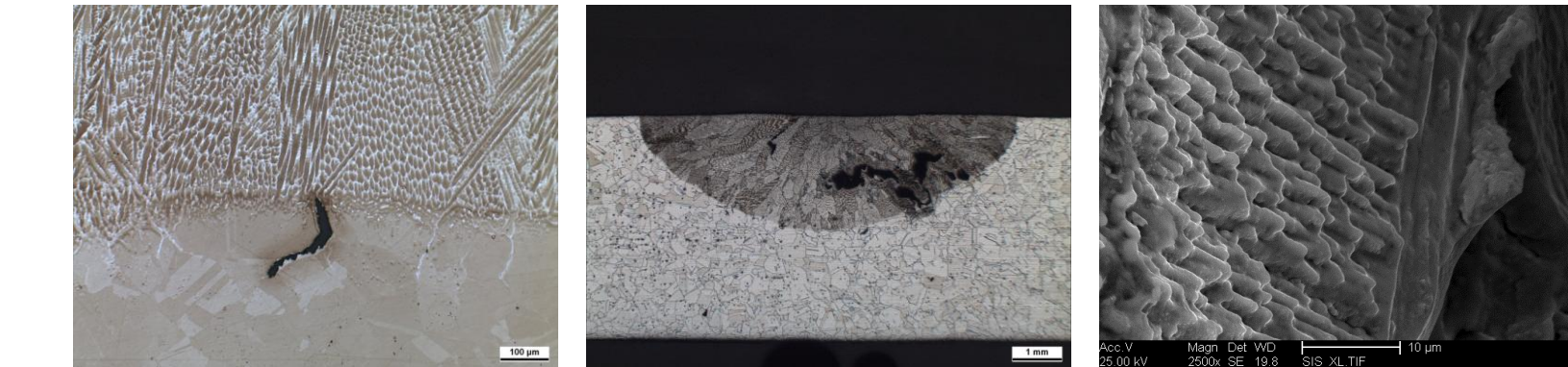
Micrographs of hot cracks in welds after PVR-test
