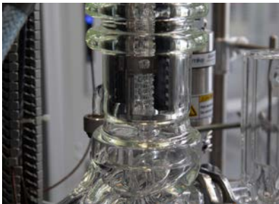
Close-up of sump outlet of SPE
