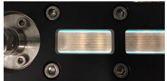
Microstructured heat exchanger used for fouling experiments - view of the microchannels
