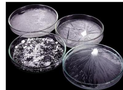
Crystallization of sodium acetate ( $\text{CH}_3\text{COONa}$ )
