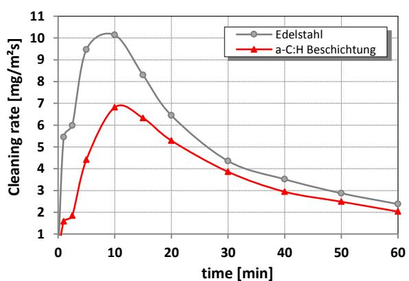
Cleaning curve of whey protein fouling on stainless steel and DLC surfaces
