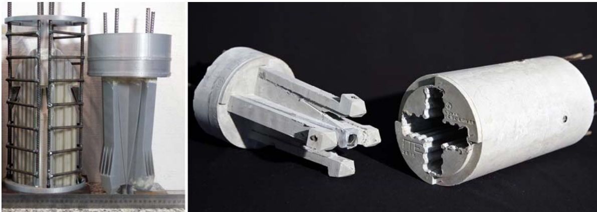
Figure 7: Molds of a column-column connection before assembling including tig-welded reinforcement cages (left); column-column connection with a snap-fit made of UHPC (right) [sources: Ledderose]
