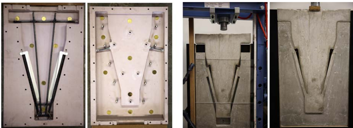
Figure 5: The two CNC-milled molds for a slab-slab connection (left); Joining of the cast connection in a testing machine (right) [sources: Ledderose]
