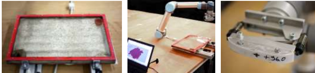
Figure 4: pellucid mould (left), setup with robot (middle), end effector with magnets M1 (right)
