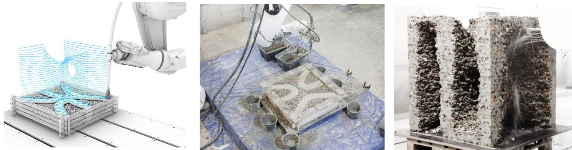
Figure 1: First Large Particle 3D Concrete Printing prototype produced at the Digital Building Fabrication Laboratory at Technische Universität Braunschweig
