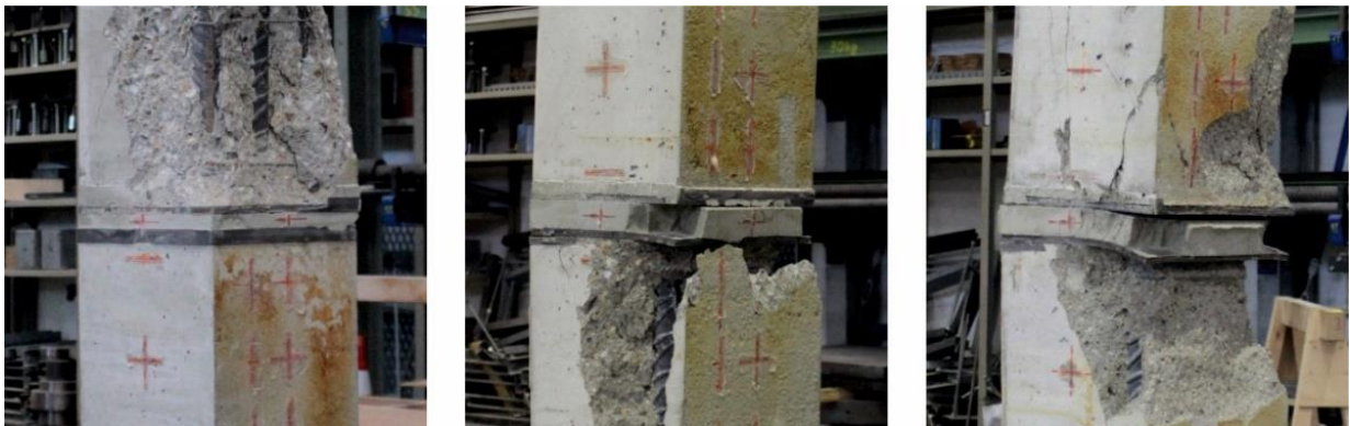
Figure 9-5: Test specimens after failure: S 9.2 (left), S 9.3 (middle) and S 9.6 (right)
