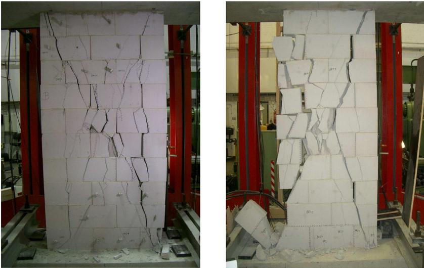
Fig. 4-31: Crack pattern, Left: Wall 3, Right: Wall 4 [Budelmann et al. 2004]
