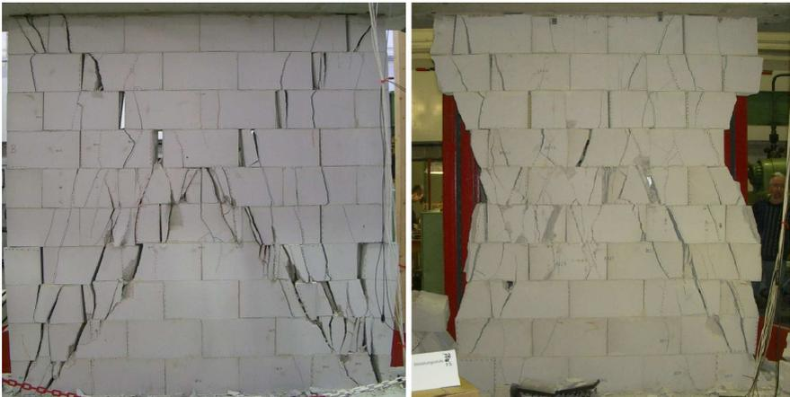
Fig. 4-28: Crack pattern, Left: Wall 1, Right: Wall 2 [Budelmann et al. 2004]
