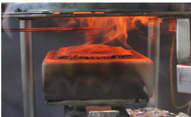
Test in installed condition under radiant heater
