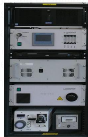
View of the FTIR gas analysis unit
