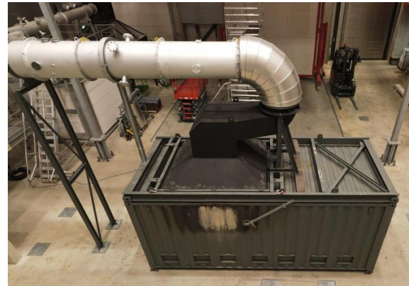
View of container calorimeter, with fire room, hood and exhaust pipe with measurement section
