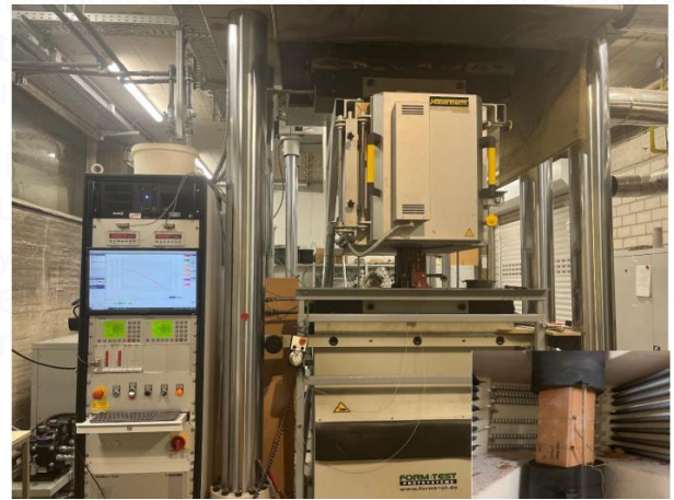
View of the high temperature compressive stress unit and a built-in specimen including temperature- and deformation equipment (bottom right)
