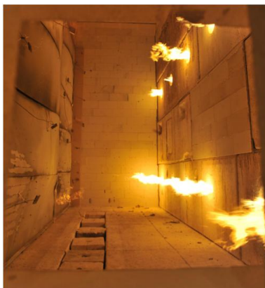
Fire test on a mechanically unloaded wall structure made of sandwich panels
