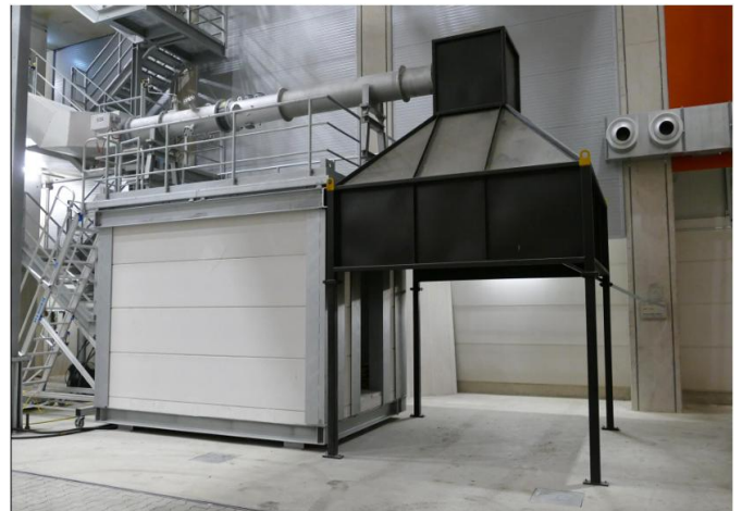
View of the Room Corner test room, consisting of a test chamber, hood, and extraction pipe with measuring equipment
