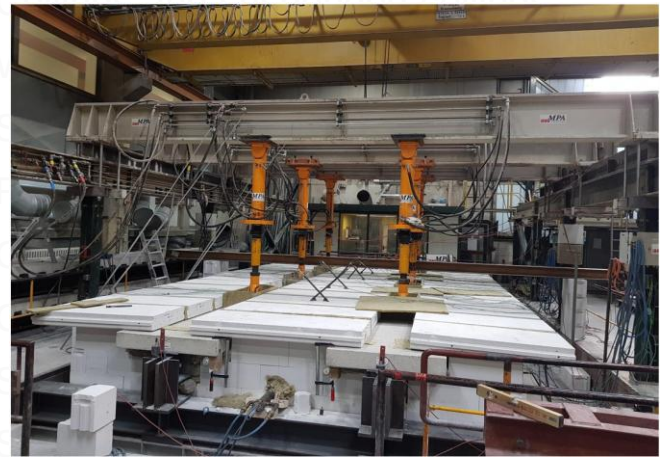
Fire test on mechanically loaded steel beams
