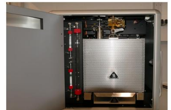
View of the CHNS analyzer and the oxygen analyzer (O 2 )
