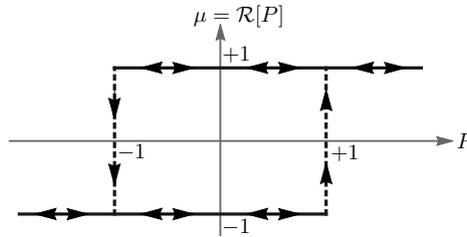
FIGURE 3. The relay operator  $\mathcal{R}$  describes the hysteresis of phase interfaces in the macroscopic scaling limit.
