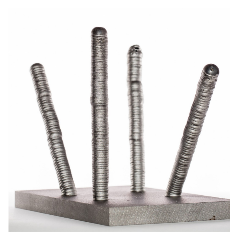
Right: Inclined WAAM steel bars for use as 3D-anchoring element in cast concrete
