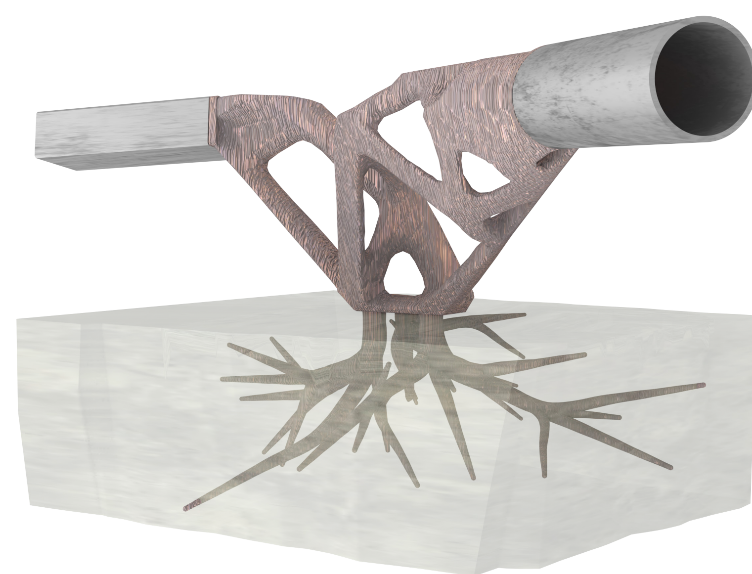
Final WAAM demonstrator. Connection of semi-finished steel products and 3D-anchoring element in cast concrete. Case study demonstrators a) connection between different cross sections and diameters b) undercuts in building direction c) intersection of bars d) variable wall thickness in building direction.
