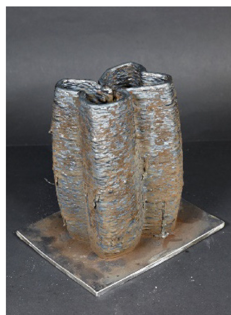
Left: WAAM component with varying cross section in build up direction
