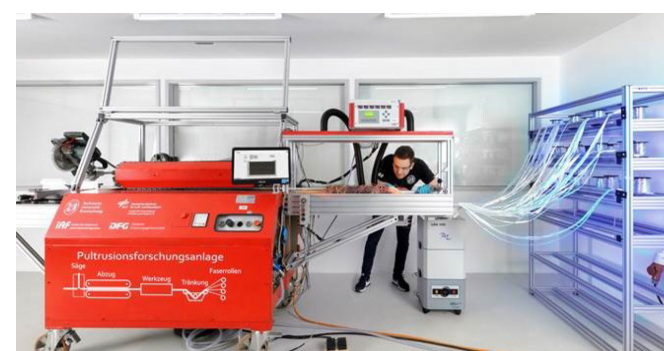
Pulltrusion of glass fiber elements, iAF
