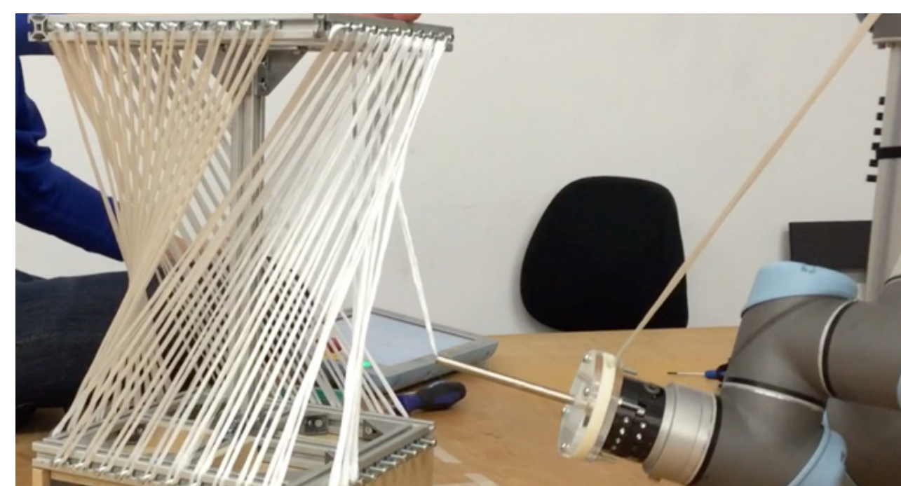
Robotic fibre winding process, developed at the Digital Building Fabrication Studio at ITE, TUBS.
