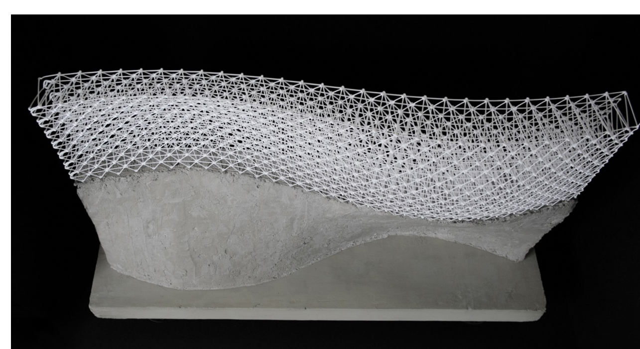
Mesh Mould, Phase 1: Spatially printed mesh, filled with concrete, Gramazio Kohler Research, ETH Zürich
