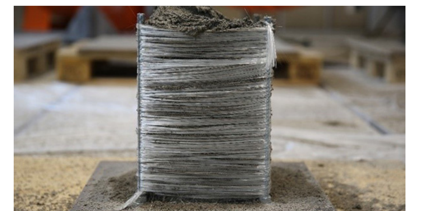
Initial test Specimen of a robotically wound stay-in-place formwork.
