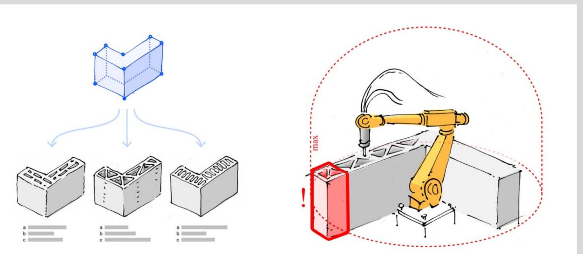
Right: Usage of FIM for steering the manufacturing process. Left: Different variants of FIM for one BIM element.
