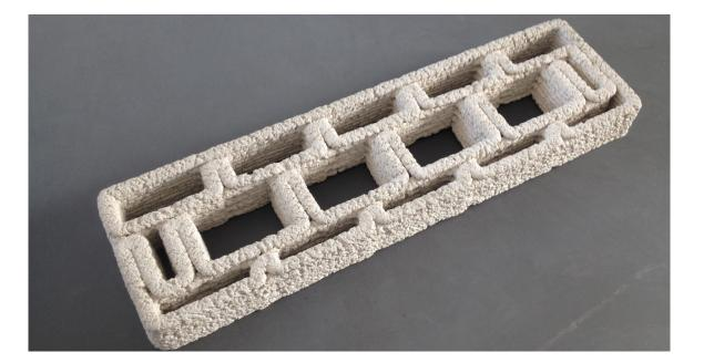
The internal structure of a concrete component produced by AM (Chair of Timber Structures and Building Construction, TUM)
