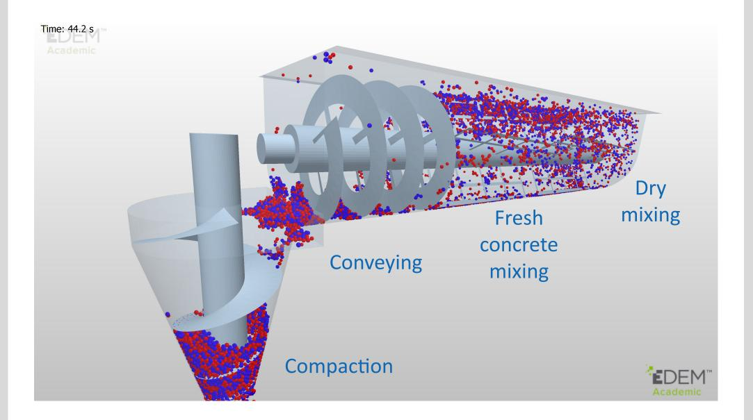
extrusion of lightweight concrete could be derived. In particular, the pumpability over greater distances poses a challenge for light aggregates due to the pressure that occurs. In general, however, good thermal conductivities and strengths can be achieved.
