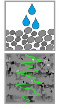
Liquid – Intrusion behaviour and interlayer bonding
