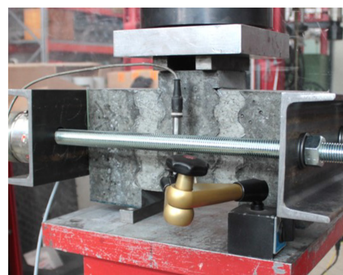
UHPC double shear test with a profiled mortar joint
