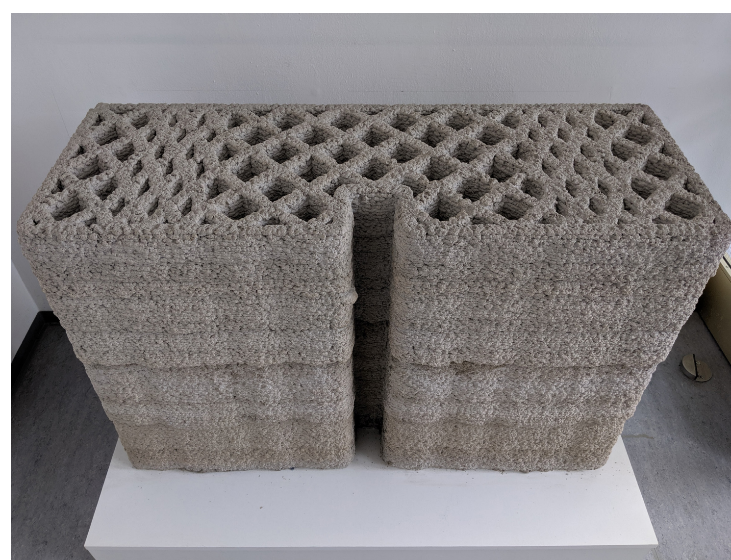
Concrete extrusion example made by the Chair of Timber Structures and Building Construction at TUM (A03).
