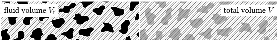
Figure 2.1.: Definition of the fluid volume V_f inside a porous medium and of the total volume V containing also the solid structure.
