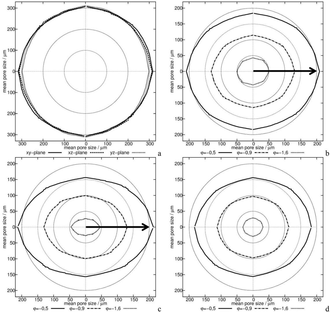
**Fig 2** Structural ellipses. **a** as received, **b** planes parallel to the rolling direction (indicated by the arrow) and the rolled surface for selected degrees of deformation, **c** planes parallel to the rolling (indicated by the arrow) direction and perpendicular to the rolled surface, **d** planes perpendicular to the rolling direction and the rolled surface
