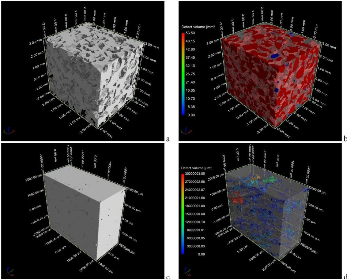
Fig 1 CT images of PA 80-110. **a** surface of the sample as received, **b** pores of the sample as received, **c** surface of the sample for  $\varphi \approx -1, 6$ , **d** pores of the sample for  $\varphi \approx -1, 6$
