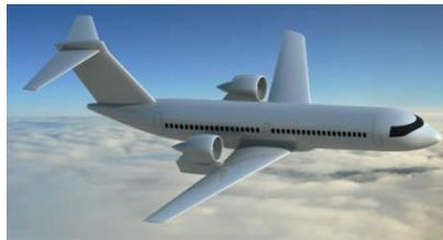
**Fig. 1** REF3 configuration for SFB 880 with over-the-wing mounted engines.
